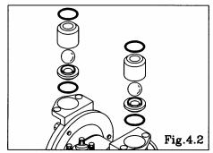
Remove the O ring, valve stopper, ball and valve seat. [Fig.4.2]
