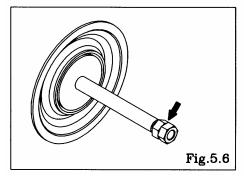
Fix a double nut to one end of the center rod and take the diaphragm and center disk off the opposite end. [Fig.5.6]
